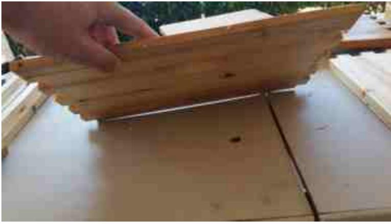
**Place top box short side handle side down. Mate top box long side with window plastic facing inside**
