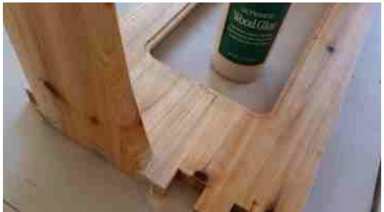
**Any stress cracks during assembly can be glued using a waterproof wood glue**
