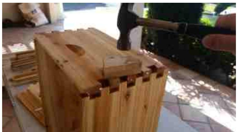
Once the dovetail joints are partially mated, use hammer and block to GENTLY finish assembly
