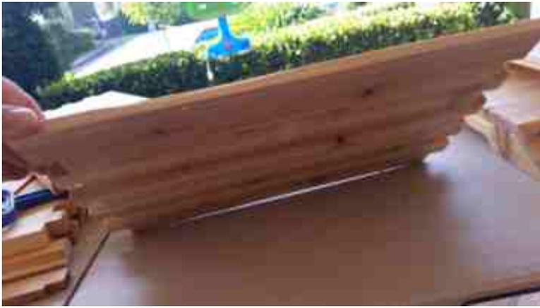
Place bottom box narrow side handle side down. Note, one of the bottom box narrow sides is shorter in height to allow for bee entrance. Make sure this shorter side is used for bottom!
